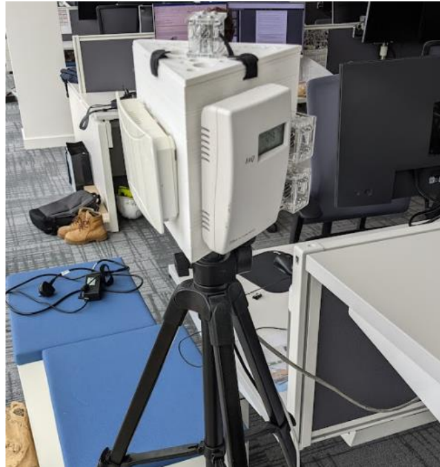
Figure 76 - Arup BPS Arc Air Quality Monitor in the Cork Office
